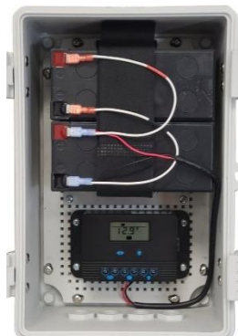
20A PWM Controller Inside
