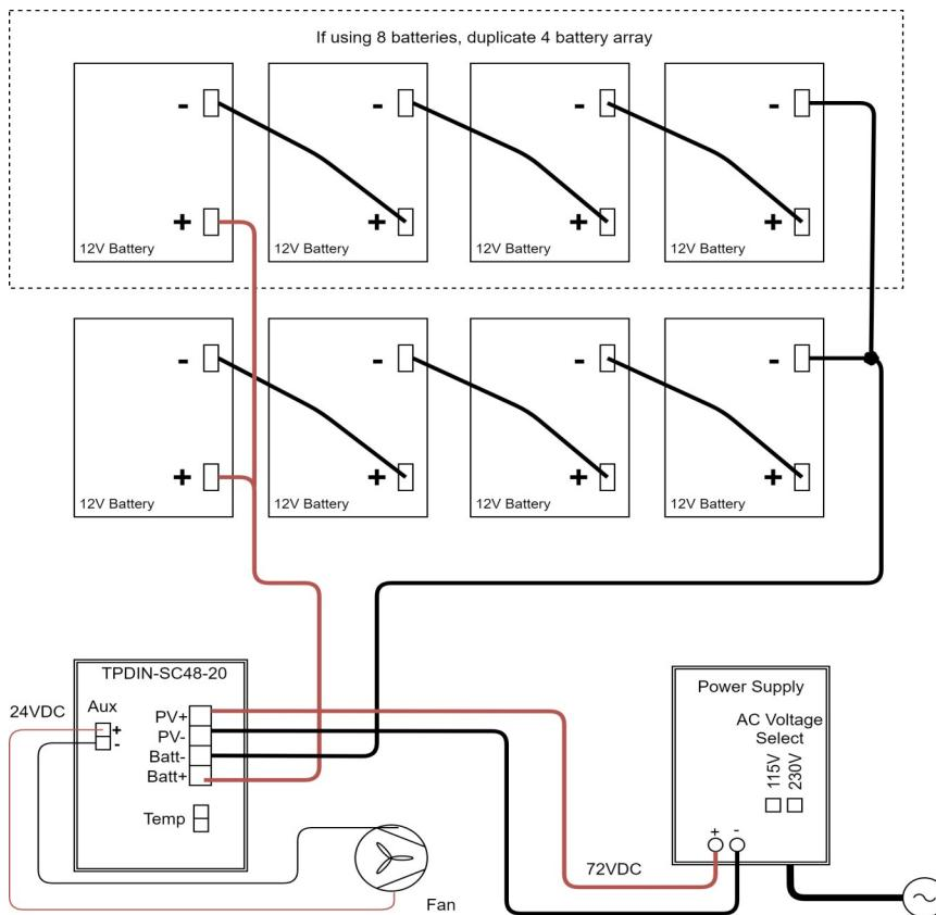
**WARNING!** The fan supplied with the system operates on 12VDC or 24VDC. It is thermostatically controlled to turn on if temperature exceeds 45C. It cannot be connected to 48V battery voltage. It can be connected to the Aux output of the controller set to 24VDC or it can be connected across one of the batteries in the array.
