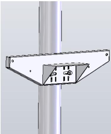
**STEP 4:** Attach The two 8mm bolts that hold the bottom bracket to the enclosure. Make sure all bolts are tight. (8-15 ft lbs)
