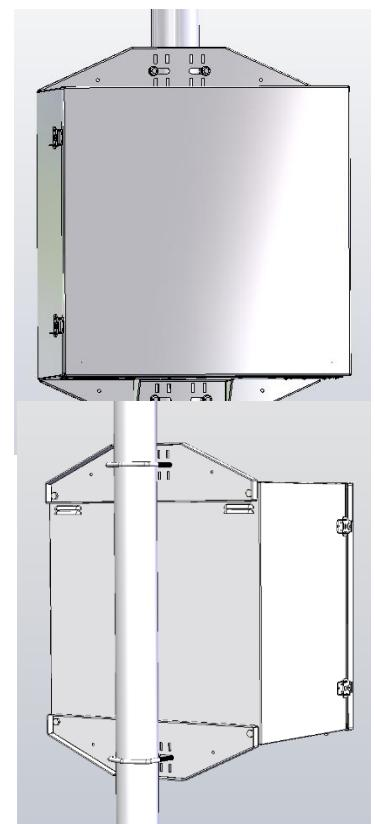
**NOTE:** The bottom plate can be removed from the enclosure if you need to add some additional feedthru. (ex; conduit connection)
