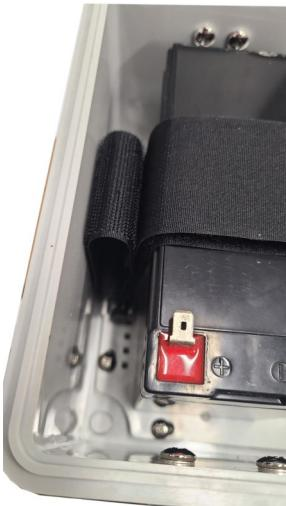
Fold the end of the strap between the battery and the enclosure wall to allow access to the end of the Velcro strap for easy removal.
