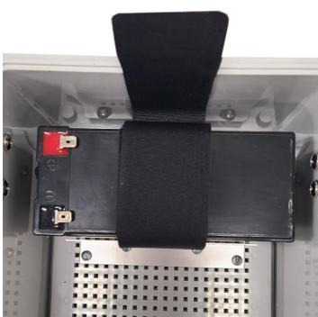
Insert the batteries by slipping under the Velcro strap and then tightening the strap.
