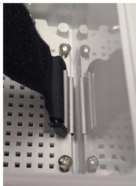
Center the bracket and attach to the mounting plate using Qty 4 #8 x 3/8 pan head self tapping screw.
