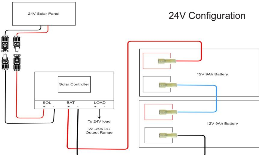
Connect the wires for any equipment, that will be powered by the system, to the controller load output on the small controller or Aux and/or PoE outputs on the large controller.
